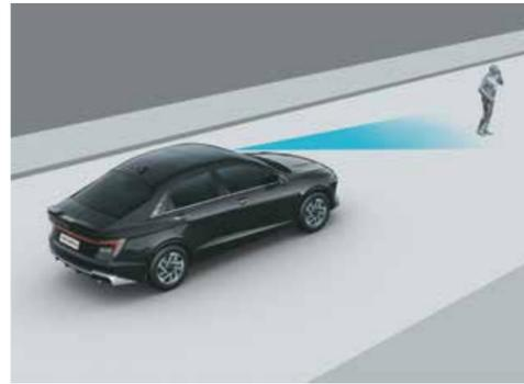
Forward Collision - Avoidance Assist - Pedestrian (FCA-Ped)
