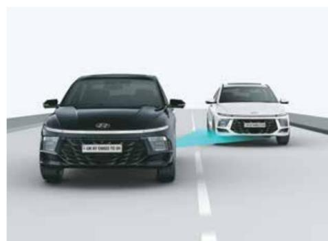
Blind-spot Collision - Avoidance Assist (BCA) & Blind-spot Collision Warning (BCW)
